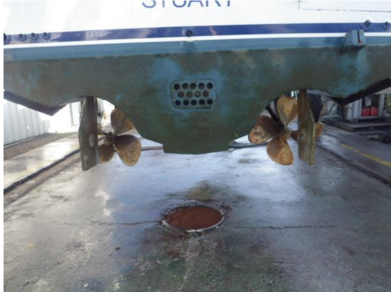
Port strut top corrosion
